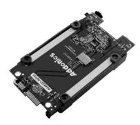
**Step 4** Turn over the PCB and secure the hard drive to the PCB with the mounting screws that come with the kit.
